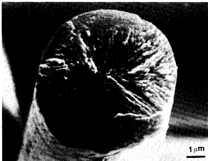
Fig. 10. SEM photo of unstabilized PBO fiber carbonized at 2000°C.
