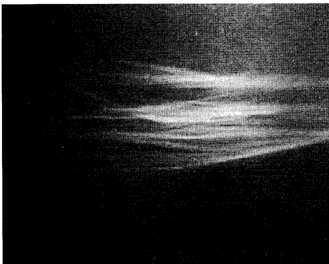
Figure 8. Spread Kevlar tow (1.6×magnification).
