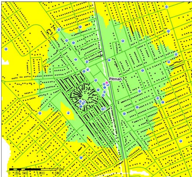
Figure 9. Pitman Station (NJ-3 & NJ-3b). Walking accessibility (1/2 mile) is depicted in green, 1 mile accessibility is depicted in yellow. Housing units are depicted as black dots and index destinations are depicted as larger blue dots.
