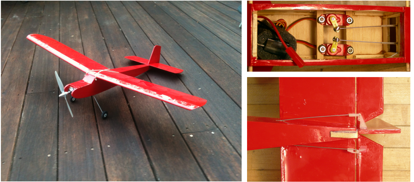
Figure 2: Left : A view of the aircraft used for testing. Top right : A view inside the fuselage (directly under the wing) where the servos which control the tail control surfaces reside; the servos (center) are connected to the tail surfaces by piano wire (center to right; the front of the plane is to the left in the image). Bottom right : A view from underneath of the tail, showing how the servo control rods attach to the elevator and rudder control surfaces.
