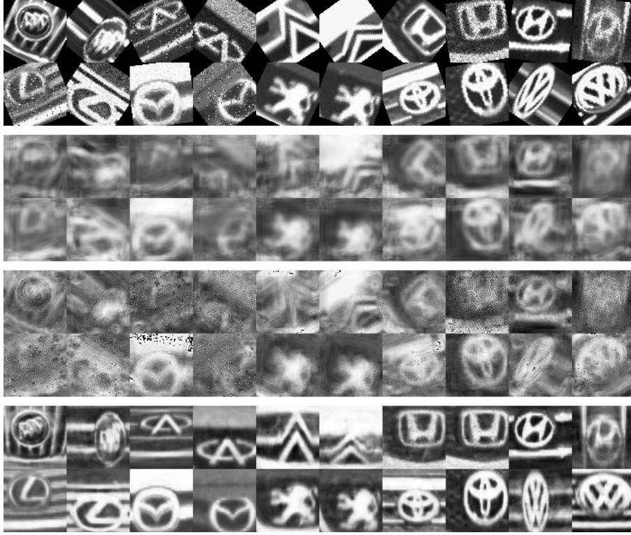
Fig. 8 The rotation restoration result of the Joint-CNN-Net, Joint-RED-Net and Joint-Cap-Net when the images are randomly rotated up to 40^\circ .
