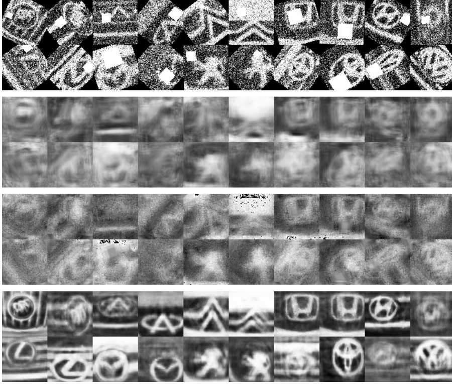
Fig. 10 The restoration result of the Joint-CNN-Net, Joint-RED-Net and Joint-Cap-Net with combined Gaussian noise, rotation and occlusion.
