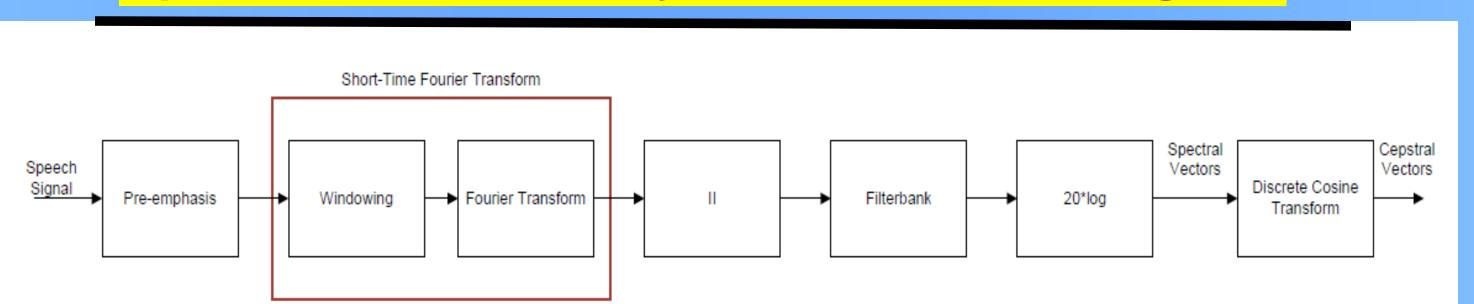
The flow block diagram is a modular representation of a cepstral-based speaker identification system. This diagram is used as a sketch of the components that needed to be implemented into a MATLAB program.
