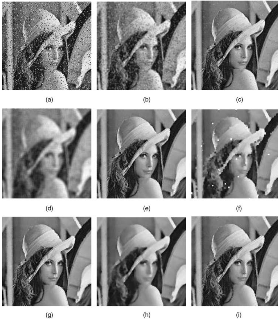
Fig. 1. Translation-invariant and spatially-variant denoising. (a) Noisy image. (b) Translation-invariant mean filter using a 3 \times 3 window. (c) Spatially-variant mean filter using a 3 \times 3 window for noisy pixels only. (d) Translation-invariant mean filter using a 7 \times 7 window. (e) Spatially-variant mean filter using a 7 \times 7 window for noisy pixels only. (f) Translation-invariant alternating filter using the 3 \times 3 square SE. (g) Spatially-variant alternating filter. (h) Translation-invariant median filter using the 5 \times 5 square SE. (i) spatially-variant median filter.
