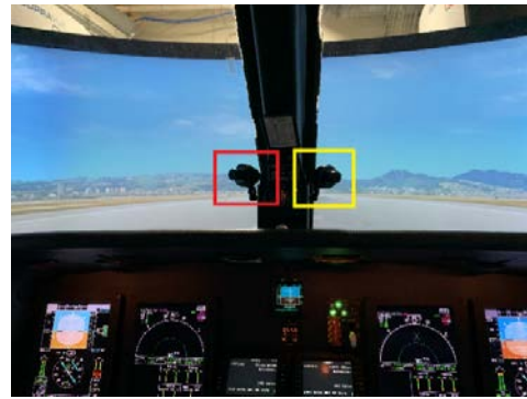
Figure 5a. Camera mounting positions for collecting data for the FAA Simulator Dataset. The box on the left was used to collect copilot data and the box on the right was used to collect pilot data.
