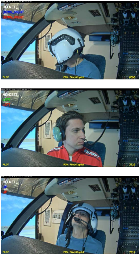
Figure 29. Pilot frames correctly classified by simulator models. The white text in the top left is the prediction of the headgear classifier. The green/blue text and red text are the nine class head pose predictions for the headset/helmet model and combined model respectively. The yellow text at the bottom displays the helicopter side prediction, prediction point of view, and frame number.
