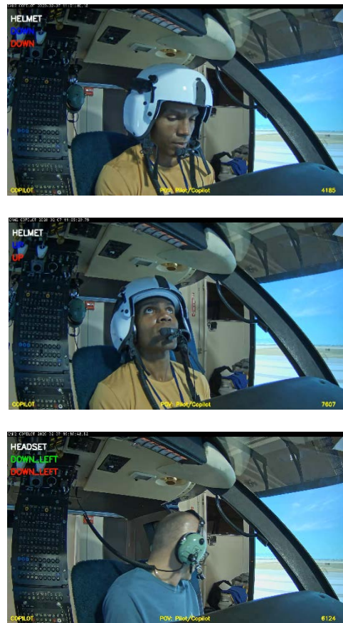
Figure 30. Copilot frames correctly classified by simulator models. The white text in the top left is the prediction of the headgear classifier. The green/blue text and red text are the nine class head pose predictions for the headset/helmet model and combined model respectively. The yellow text at the bottom displays the helicopter side prediction, prediction point of view, and frame number.
