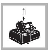
**10.** Place the blank into the cell holder and close the light shield.
