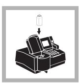
12. Place the prepared sample into the cell holder. Close the light shield. Results in platinum-cobalt units will be displayed.
