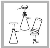
**2.** Assemble the filtering apparatus (0.45 micron membrane filter, filter holder, filter flask, and aspirator). NCASI prescribes a 0.8 micron filter.
