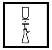
**5.** Turn off the vacuum and lift off the funnel top. Using sterile forceps, transfer the filter to the previously prepared petri dish.
