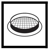
**6.** With a slight rolling motion, place the filter, grid side up, on the absorbent pad. Check for trapped air under the filter and make sure the filter touches the entire pad. Replace the petri dish lid.
