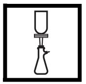
**4.** Shake the sample vigorously to mix. Pour 100 mL of sample or diluted sample into the funnel. Apply vacuum and filter the sample. Rinse the funnel walls three times with 20 to 30 mL of sterile buffered dilution water.
