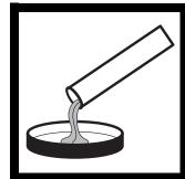
**2.** Invert ampules two or three times to mix broth. Break open an ampule of m-ColiBlue24 Broth using an ampule breaker. Pour the contents evenly over the absorbent pad. Replace the petri dish lid.
