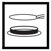
**1.** Use sterilized forceps to place a sterile, absorbent pad in a sterile petri dish. Replace the lid on the dish.
