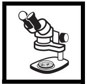
**8.** Remove the petri dish from the incubator and examine the filters for colony growth. Colonies are typically readily visible; however, a stereoscopic microscope or other 10–15X magnifier may be useful. Red and blue colonies indicate total coliforms and blue colonies specifically indicate *E. coli*.
