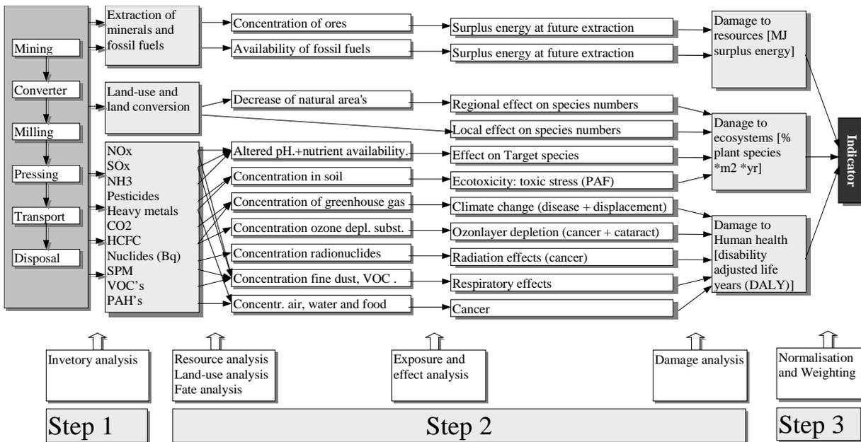
Figure 7: Detailed representation of the damage model (step 2)
