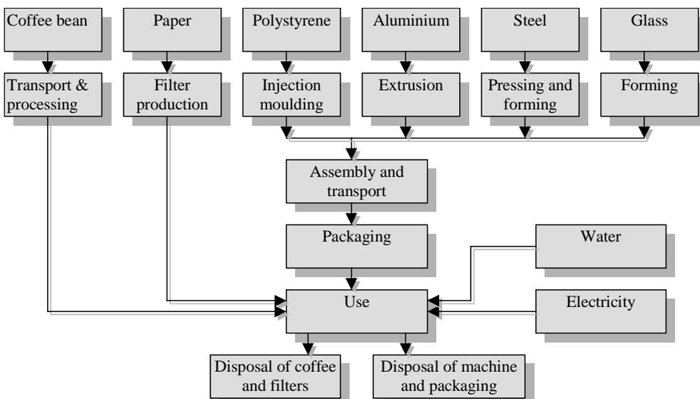
Figure 2: Example of a simplified process tree for the life cycle of a coffee machine.
