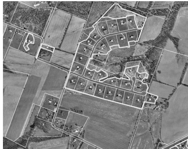
Figure 2. Housing Centroid Automation. This image depicts an orthophoto of one newly developed housing tract. The thick lines delineate the “patches” of new urban growth as classified by the land-use/land-cover dataset. The thin lines delineate the property parcel lines. The target symbol denotes the automated centroid location estimated for each new housing unit. Sprawl measurements are calculated for each housing-unit centroid.
