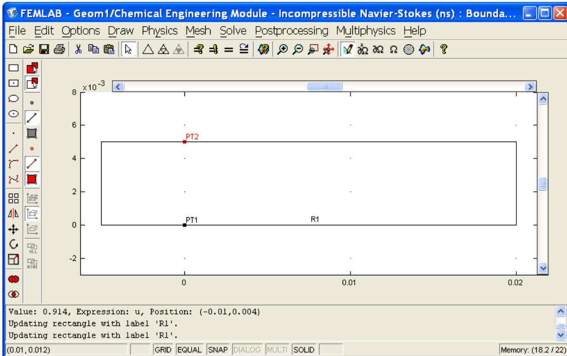
11. Calculate the boundary layer thickness  $\delta = \frac{5.0x}{\sqrt{N_{Re,x}}} = 5.0 \sqrt{\frac{\mu x}{\rho v_\infty}}$  where  $x = 0.02$  m. Then increase the gridding within the boundary layer region.
