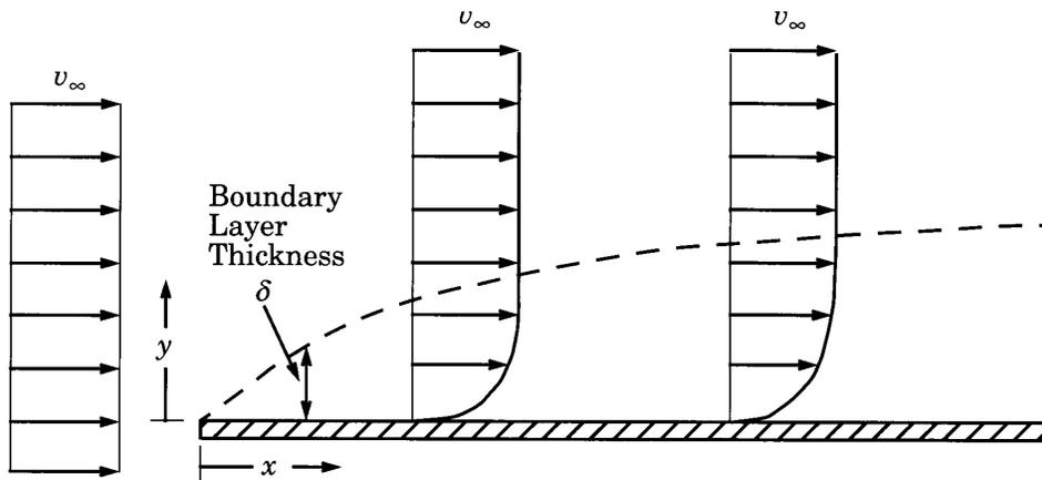
Figure 5-10 Laminar Boundary Layer for Flow Past a Flat Plate
