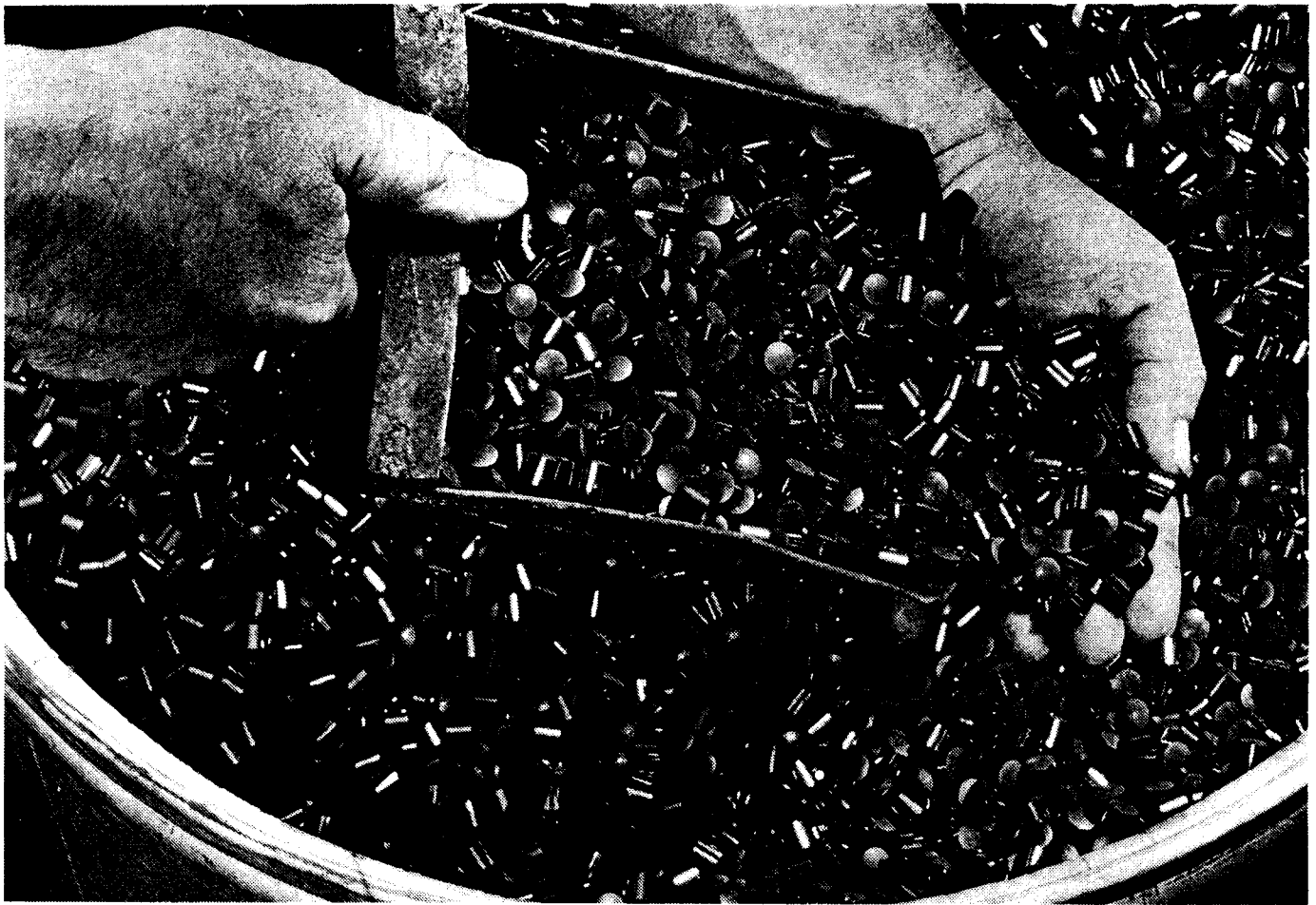
Figure 4.1 High-temperature water-gas shift catalyst, iron oxide promoted with chromia; 5 × 5-mm pellets. (Courtesy of United Catalysts Inc., Louisville, Ky.)
