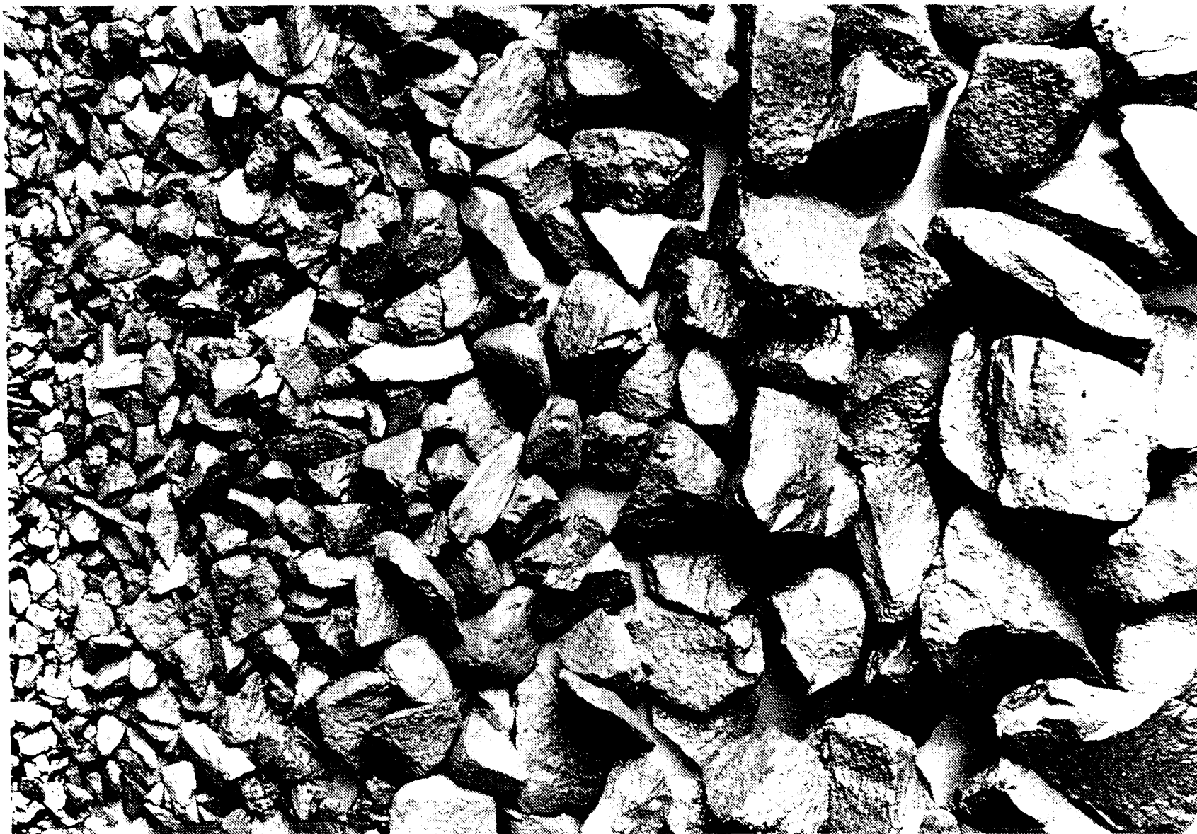
Figure 4.12 Topsøe ammonia-synthesis catalyst KMI. The three sizes are about 1.5 to 3 mm, 6 to 10 mm, and 12 to 21 mm. (Courtesy of Haldor Topsøe, A/S, Copenhagen, Denmark)
