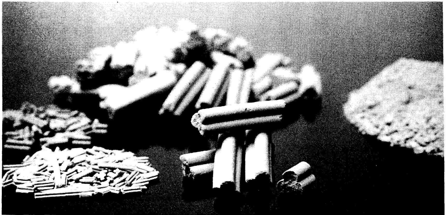
Figure 4.4 Extrudates of different sizes with a trilobal cross section, termed Trilobes®. Note the shadows. (Courtesy of American Cyanamid Company)
