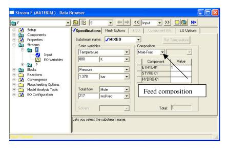
11. To input the reactor specifications, double click on the reactor block. The reactor *Data Browser* opens. You can input values for pressure, temperature, heat duty, vapor fraction (You need to input values for only two variables –Use the drop down list). For an isothermal reactor specify the outlet temperature and for the adiabatic
