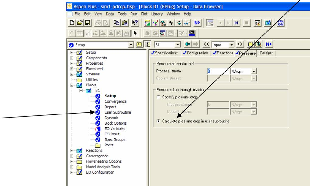
18. Next select the User Subroutine entry in the data browser. Supply the name of the function as ‘ERGUN’. The user subroutine requires two catalyst parameters for its calculations. The first parameter is particle diameter in units of meters and the second parameter is catalyst bed void fraction. Select 4.7 mm for your particle size and 0.445 for your void fraction.
