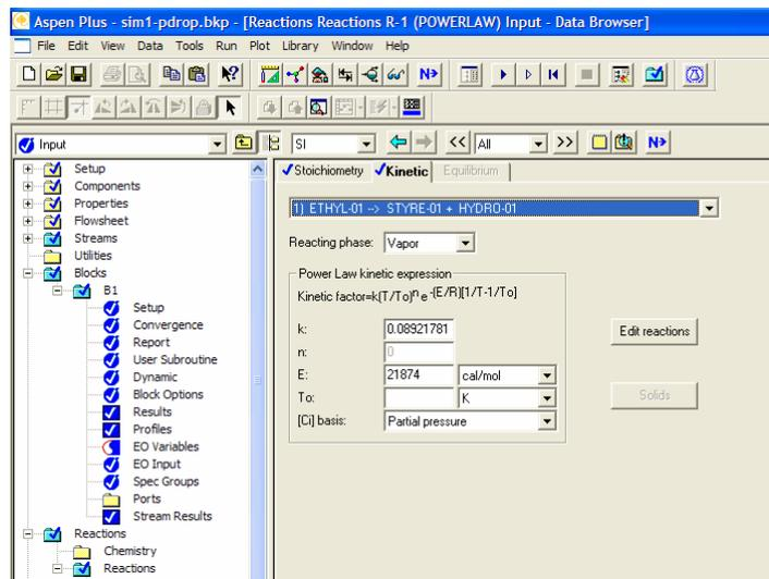
20. Go back to reactor specification, Reactions tab, and select this reaction set.
