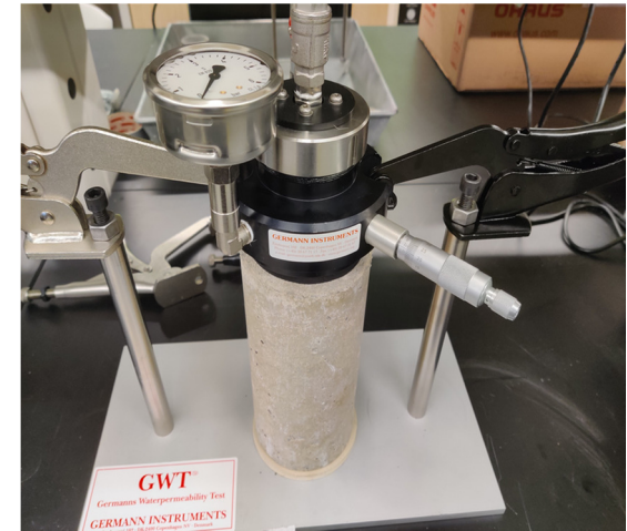
German's water permeability test
