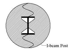
Figure 5. Sample Impact Attenuator. Impact attenuators surround posts, creating a larger surface area for impact as well as protecting motorcyclists from the sharp edges of posts (Adapted from FEMA, 2000).
