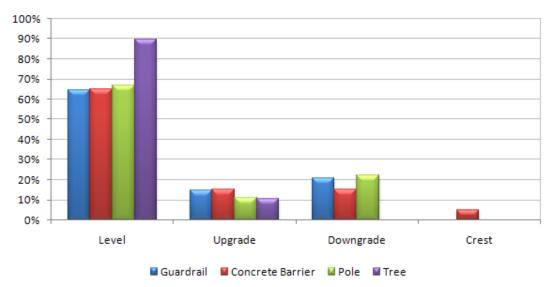
Figure 52. Grade of road at crash sites by collision type.
