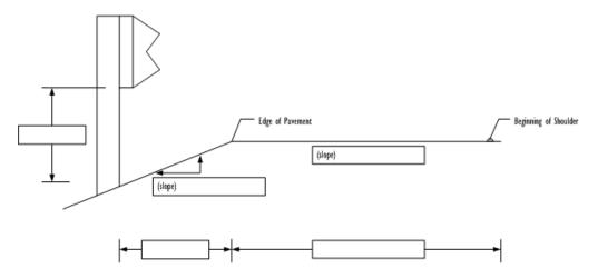
Figure 43. Guardrail and Road Environment Measurements. This figure was included in the site survey sheets to gather data about the distance of the object from the road and the slope of the road.
