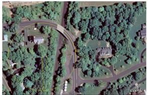
Figure 41. Example radius of curvature measurement from Google Earth Pro. This collision occurred in Mercer County on Route 640. The radius of curvature is 200 feet.
