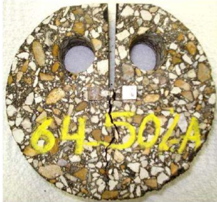
Figure 3-3. DCT Test Specimen after Test
