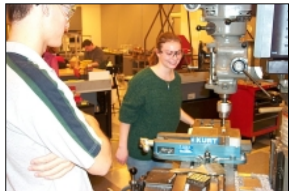
Figure 3: Fabricating connecting rod with milling machine.
