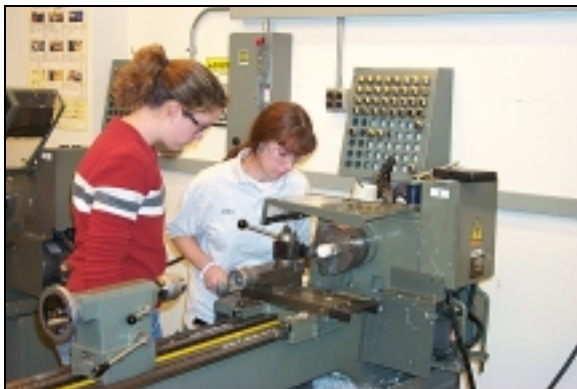
Figure 2: Turning o-ring grooves on a piston.
