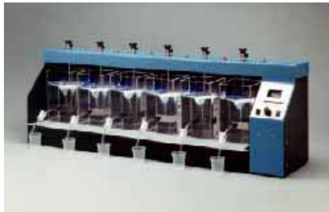
Figure 2: Jar Testing Apparatus 2
