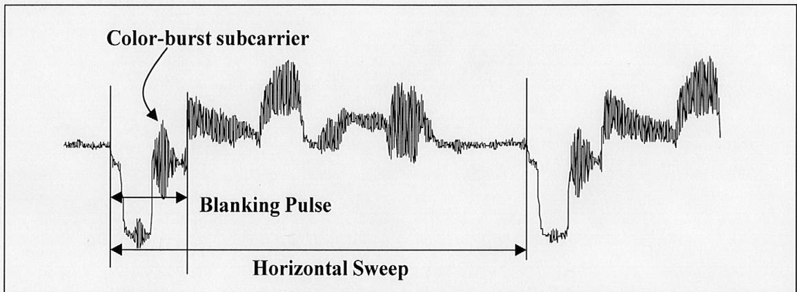
**Figure 2** Composite NTSC baseband video signal
