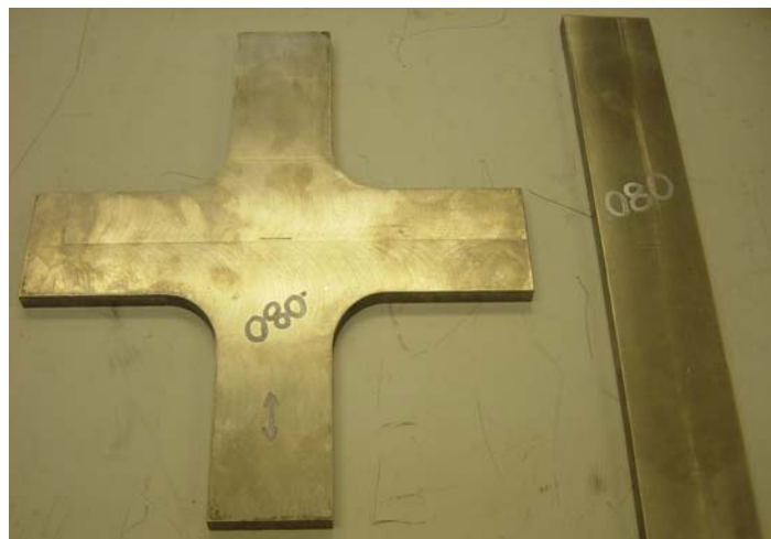
Figure 4.2: Test specimens for AE inspection with biaxial and uniaxial loading.
