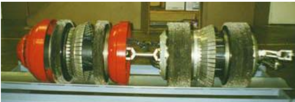
Figure 2.5: MFL inline inspection tool: the “Pig”.
