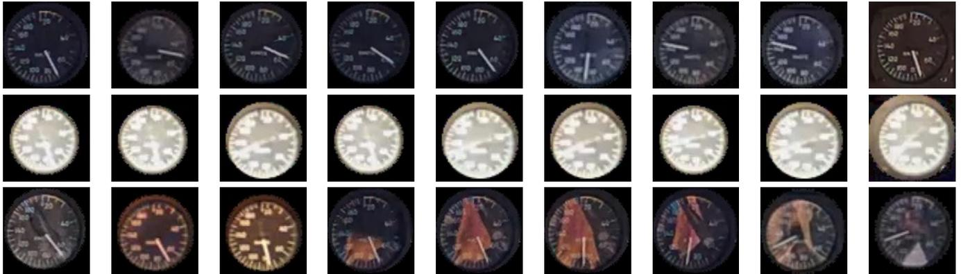
Fig. 3. 1<sup>st</sup> Row: Airspeed gauge images without glare, sun light distortion or varying ambient lights. 2<sup>nd</sup> Row: Airspeed gauges under challenging night light conditions. These frames have low readability even with an expert human eye. 3<sup>rd</sup> Row: Airspeed gauge images with different glaring and ambient effects.
