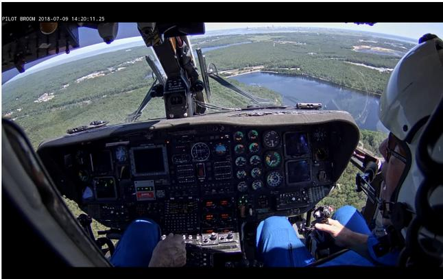
Fig. 4. A sample camera view of the instrument panel that contains the different gauges. Each gauge displays the value of a flight parameter.
