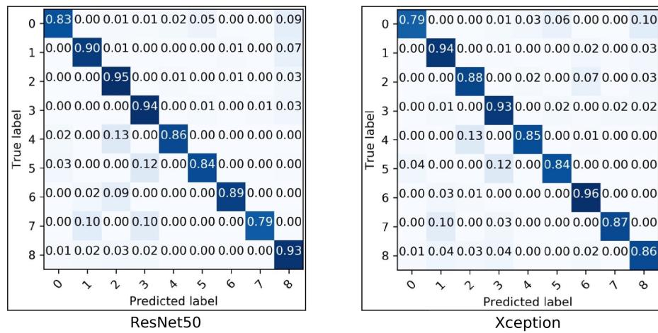
**Figure 6.** Normalized confusion matrices for 2 CNN architectures with cockpit information dataset, i.e., ResNet50, and Xception.
