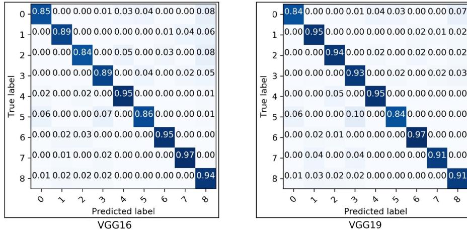
**Figure 5.** Normalized confusion matrices for 2 CNN architectures with cockpit information dataset, i.e., VGG16, VGG19.
