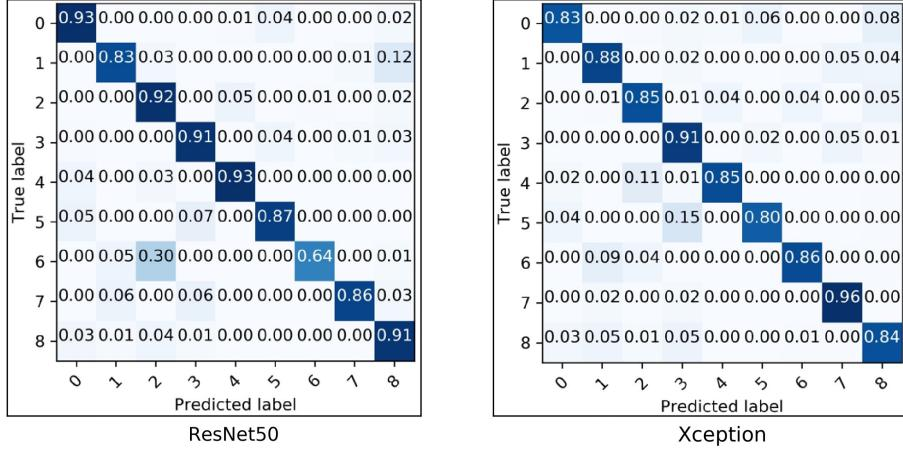
**Figure 8. Normalized confusion matrices for 2 CNN architectures without (i.e. masked out) cockpit information dataset, i.e., ResNet50, and Xception.**
