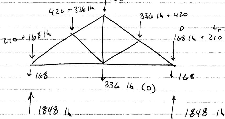
CONTROLLING LOAD COMBINATION FOR TENSION
