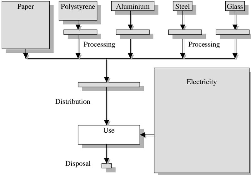
Figure 4: The coffee machine process tree, where the size of the process blocks is proportional to the relative importance of the process.
