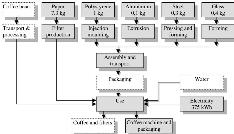
Figure 3: Process tree of a simplified coffee machine model with amounts and assumptions. White boxes are not included in the analysis.
