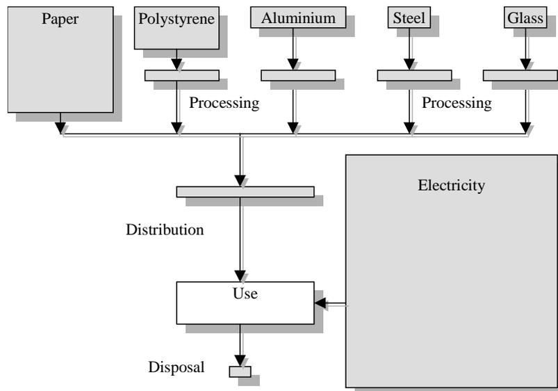
*(graphical representation of the results of an Eco-indicator analysis of a coffee machine; the size of the boxes indicates the relative contribution to the environmental load)*
