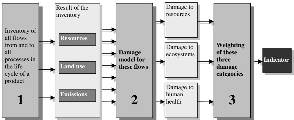
Figure 6: General procedure for the calculation of Eco-indicators. The light coloured boxes refer to procedures, the dark coloured boxes refer to intermediate results.
