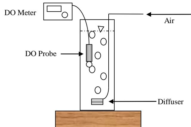
The transfer of oxygen takes place through the bubble gas-liquid interface. If the gas inside the bubble is air, and an oxygen deficit exists in the water, the oxygen transfers from the bubble into the water. Most gases are only slightly soluble in water; among these are hydrogen, oxygen and nitrogen. Solubility is influenced by many variables such as the presence of impurities and temperature.
