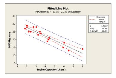
**FIGURE 16.7**: The fitted straight line to the highway mpg versus engine capacity data of Table 12.5 (leaving out the two "inconsistent" data points) along with the 95% confidence interval (long dashed line) and the 95% prediction interval (short dashed line). (Again, the additional terms—S, R-Sq, and R-Sq(adj)—are discussed later.)
