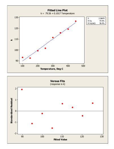
**FIGURE 16.8**: Modeling the temperature dependence of thermal conductivity. Top: fitted straight line to the thermal conductivity (k) versus temperature  $(T^{\circ}C)$  data in Table 16.6; Bottom: standardized residuals versus fitted value,  $\hat{y}_i$ .
