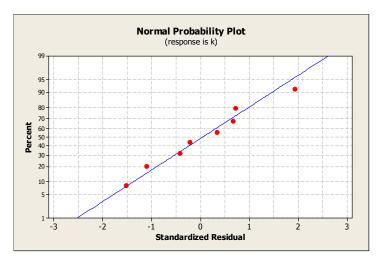
**FIGURE 17.4**: Normal probability plot for the residuals of the regression analysis of the dependence of thermal conductivity, *k*, on temperature in Example 16.5. The postulated model, a two-parameter regression model with Gaussian distributed zero mean errors, appears valid.
