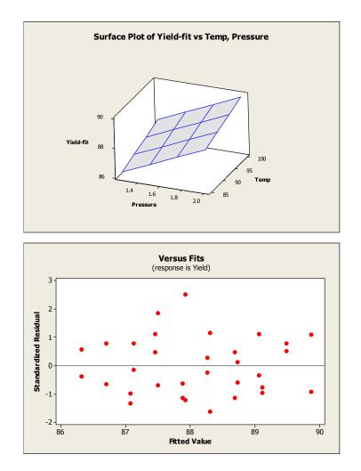
**FIGURE 16.11**: Catalytic process yield data of Table 16.1. Top: fitted plane of yield as a function of temperature and pressure; Bottom: standardized residuals versus fitted value  $\hat{y}_i$ . Nothing appears unusual about these residuals.
